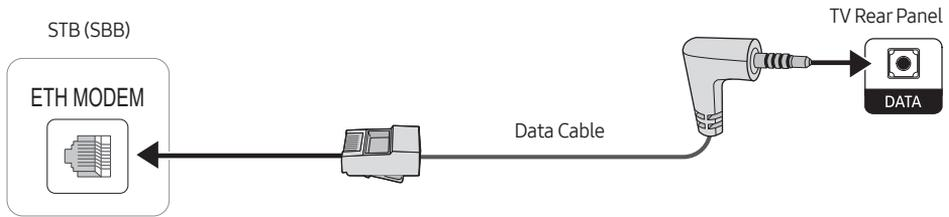
Connect the **DATA** port of the TV to the **ETH MODEM** port of the STB (SBB) with the Data cable.
